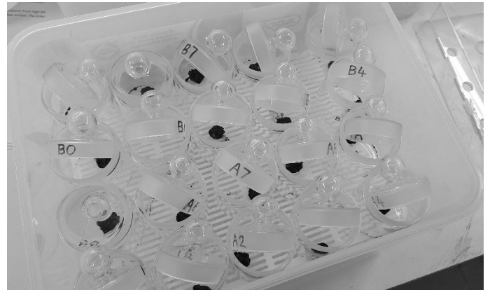
Figure 3. Batch of soil samples equalising to K 2 CO 3 solution
