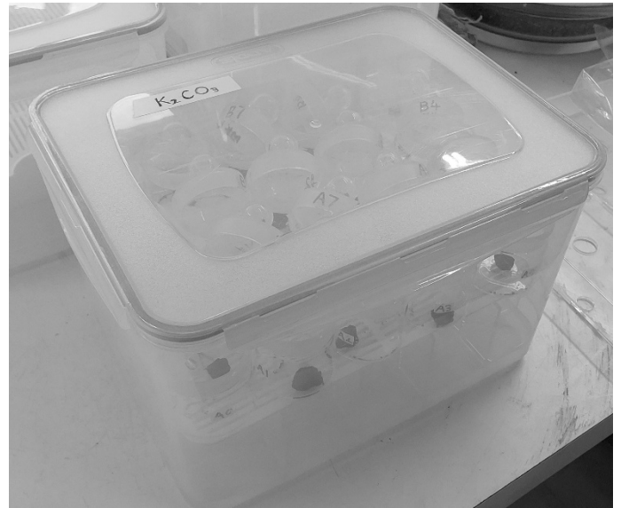
Figure 2. Airtight container with saturated K 2 CO 3 solution
