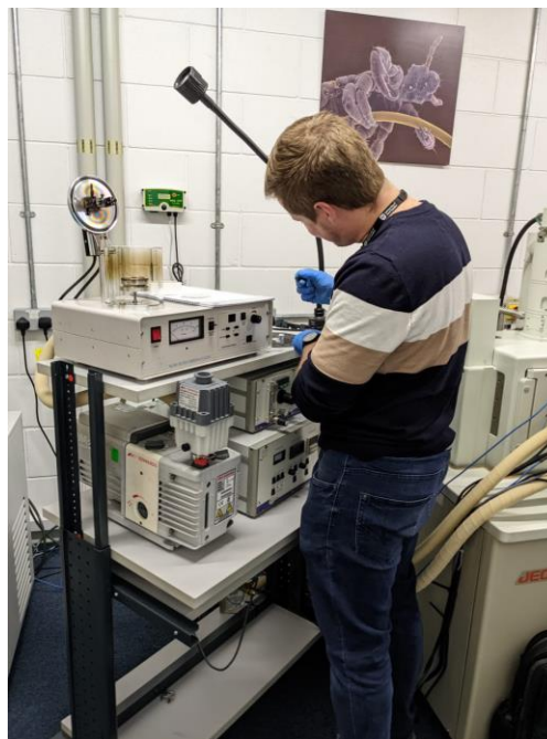
Figure 3 - Mr Waters preparing the samples through carbon coating to use in the SEM apparatus
