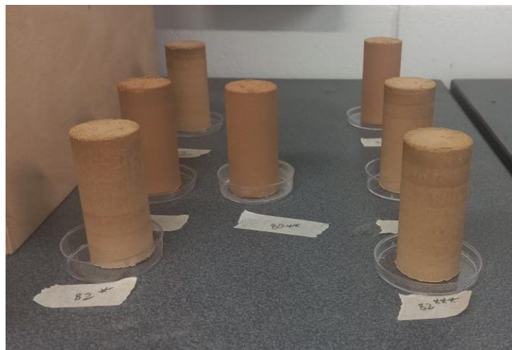
Figure 5 - Several UCS samples prepared for testing
