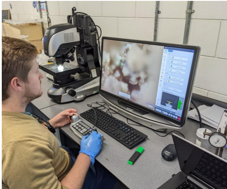
Figure 4 - Mr Waters using the 3D microscope to observe and record particle topography
