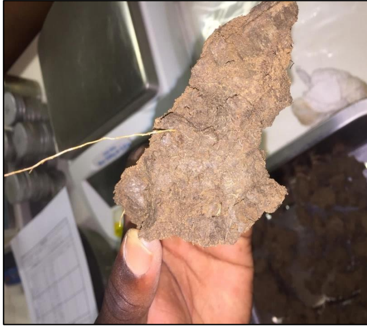
Figure 3-3: Chunk of clayey “slicken sided” soil
