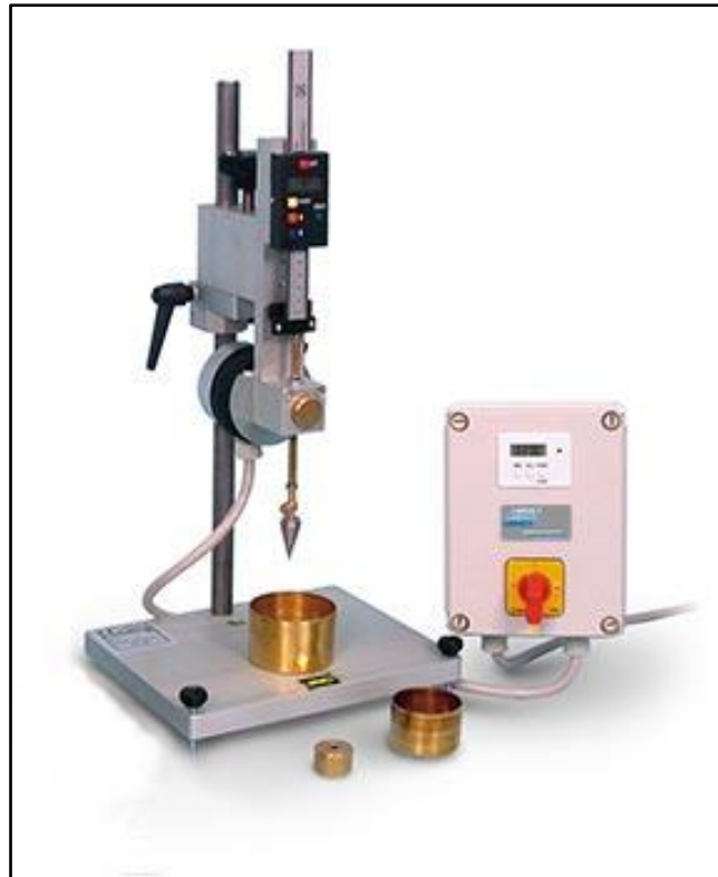
Figure 2-6: Typical BS fall-cone apparatus (BS 1377-2, 1990)
