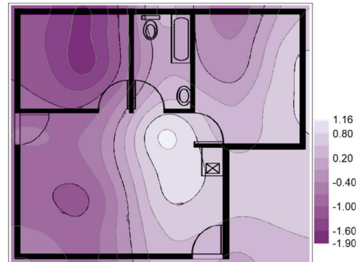
APPENDIX F - Figure 36: December Year 3 SM cavity raft foundation movement in (mm)
