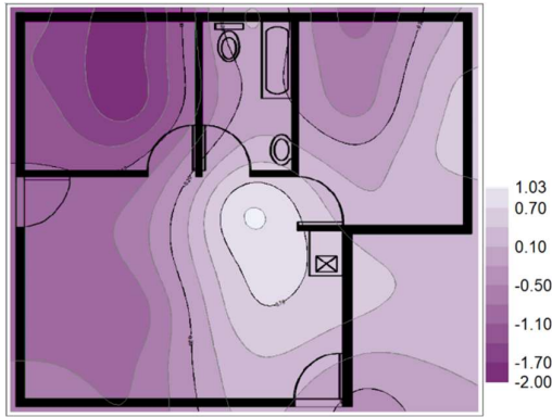
APPENDIX F - Figure 19: July Year 2 SM cavity raft foundation movement in (mm)
