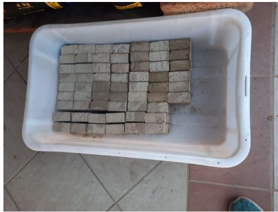
Figure 3.16: The manufacturing of scale one to six bricks
