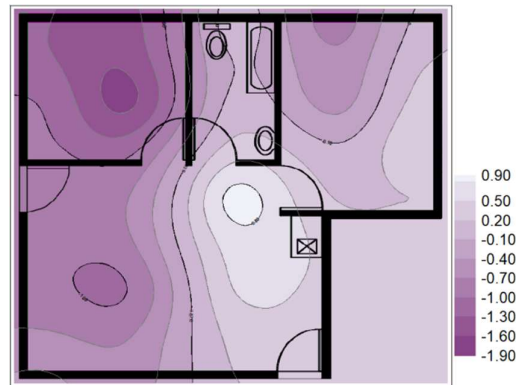
APPENDIX F - Figure 11: November Year 1 SM cavity raft foundation movement in (mm)
