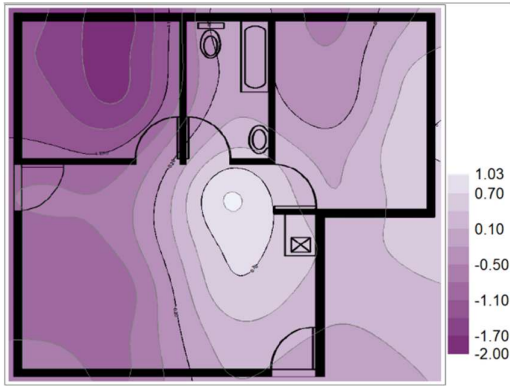
APPENDIX F - Figure 31: July Year 3 SM cavity raft foundation movement in (mm)
