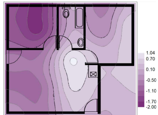
APPENDIX F - Figure 24: December Year 2 SM cavity raft foundation movement in (mm)
