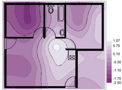
APPENDIX F - Figure 17: May Year 2 SM cavity raft foundation movement in (mm)
