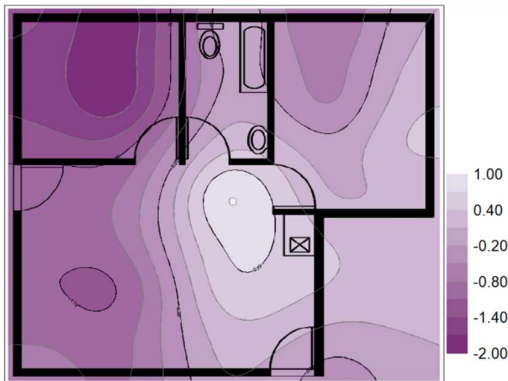
APPENDIX F - Figure 20: August Year 2 SM cavity raft foundation movement in (mm)
