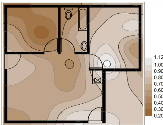
APPENDIX E - Figure 2: February Year 1 SM raft foundation movement in (mm)
