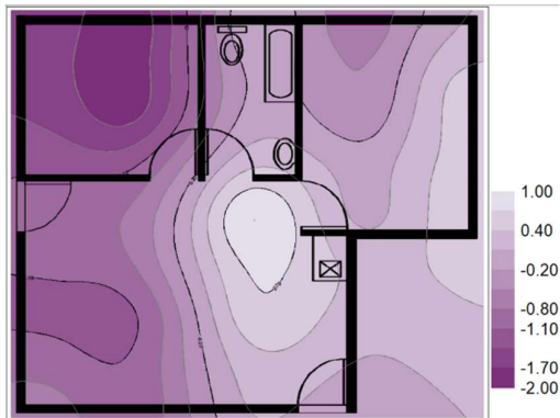
APPENDIX F - Figure 33: September Year 3 SM cavity raft foundation movement in (mm)
