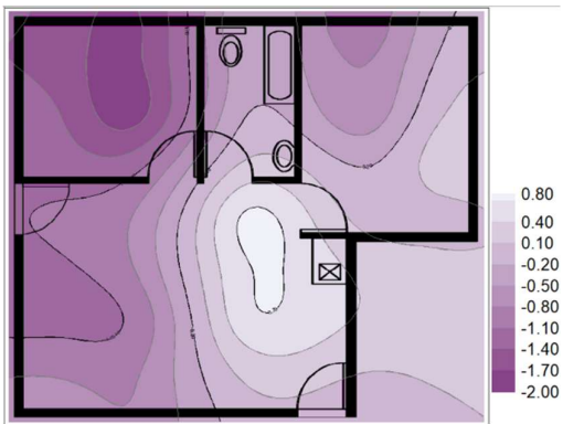
APPENDIX F - Figure 9: September Year 1 SM cavity raft foundation movement in (mm)
