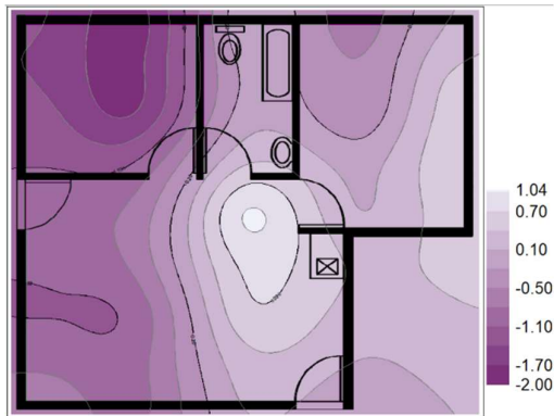
APPENDIX F - Figure 32: August Year 3 SM cavity raft foundation movement in (mm)
