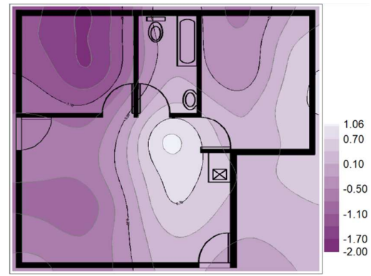
APPENDIX F - Figure 28: April Year 3 SM cavity raft foundation movement in (mm)
