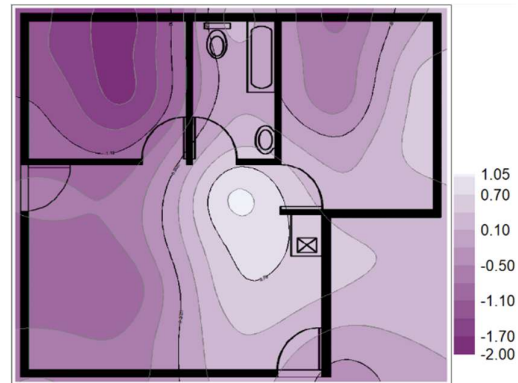
APPENDIX F - Figure 18: June Year 2 SM cavity raft foundation movement in (mm)
