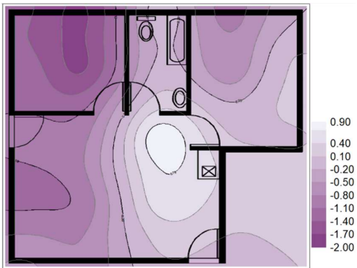
APPENDIX F - Figure 8: August Year 1 SM cavity raft foundation movement in (mm)
