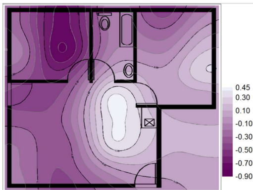
APPENDIX F - Figure 2: February Year 1 SM cavity raft foundation movement in (mm)
