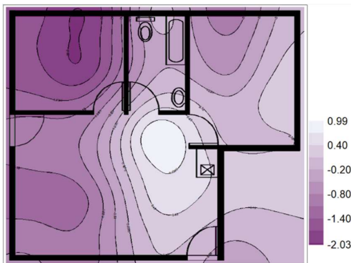
APPENDIX F - Figure 21: September Year 2 SM cavity raft foundation movement in (mm)
