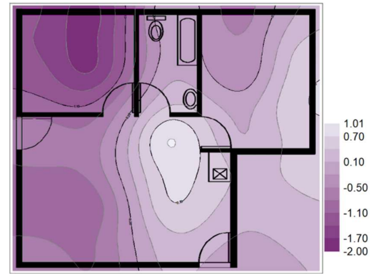
APPENDIX F - Figure 30: June Year 3 SM cavity raft foundation movement in (mm)
