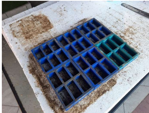
Figure 3.15: 3D-printed moulds for manufacturing bricks scaled one to six
