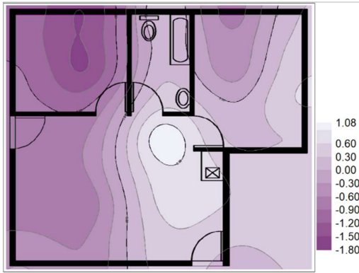
APPENDIX F - Figure 13: January Year 2 SM cavity raft foundation movement in (mm)
