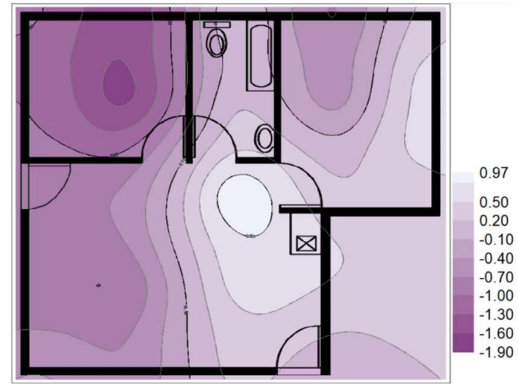
APPENDIX F - Figure 16: April Year 2 SM cavity raft foundation movement in (mm)
