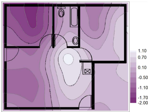
APPENDIX F - Figure 25: January Year 3 SM cavity raft foundation movement in (mm)
