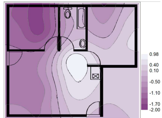
APPENDIX F - Figure 23: November Year 2 SM cavity raft foundation movement in (mm)
