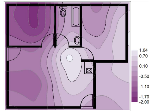
APPENDIX F - Figure 29: May Year 3 SM cavity raft foundation movement in (mm)
