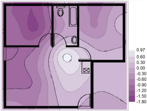
APPENDIX F - Figure 7: July Year 1 SM cavity raft foundation movement in (mm)
