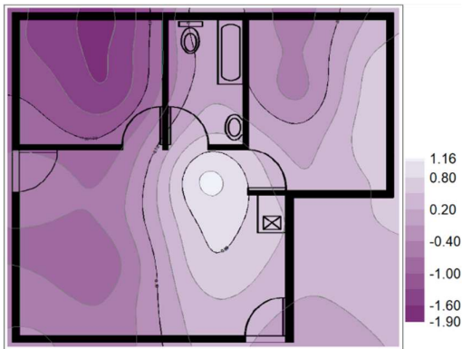
APPENDIX F - Figure 26: February Year 3 SM cavity raft foundation movement in (mm)
